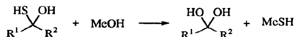
Figure 1. Isodesmic reaction for the conversion of hemi-thio acetals and ketals to the corresponding hydrate.
